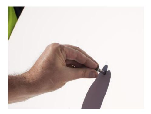
Pass four carriage bolts through the reflector.
