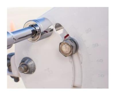
All four elevation lock down bolts need to be loosened and their four associated lock washers disengaged prior to beginning the adjustment of the elevation process.
