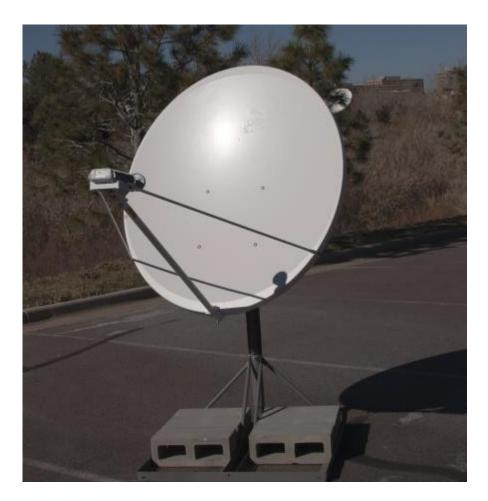
The antenna is now ready for cabling and modem installation.
