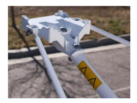
**NOTE:** The long end of the side rods attach to the reflector and the short end attaches to the TRIA Interface Casting.
