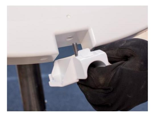
Attach the Reflector adapter casting to the reflector using a Carriage bolt and Serrated Flange Hex Nut.
