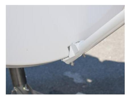
Attach the Feed support tube to the Reflector adapter casting using carriage bolts and Serrated Flange Hex nuts.
