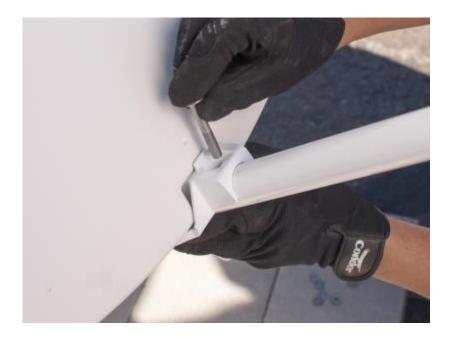
Attach the Side Rods to the TRIA Interface casting using bolts and Serrated Flange Hex nuts. Hand tighten this hardware only at this time.
