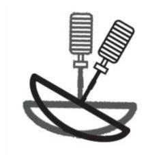
Reverse the direction of the sweep again, now sweeping to the center, and listen for the TRIA to emit the high/steady tone. The antenna is now in the center of the beam.
