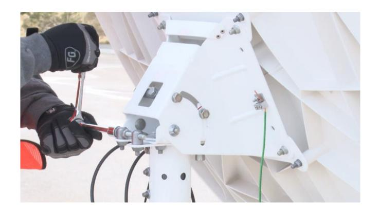
Loosen the Azimuth base plate bolts using a 17mm ratchet.
