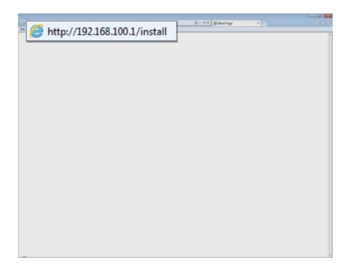
Click the forward arrow in the Address bar. The modem enters the Installation Mode.
