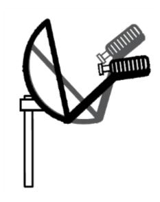
Reverse the direction of the sweep, now sweeping to raise the TRIA, and listen for the TRIA to progress through the tone sequence. Stop the sweep when the TRIA emits the low/slow tone. This is the end of the second fine-tune learning pass.
