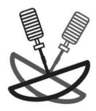
Reverse the direction of the sweep, now sweeping to the right, and listen for the TRIA to progress through the tone sequence. Stop the sweep when the TRIA emits the low/slow tone. This is the end of the second fine-tune learning pass.
