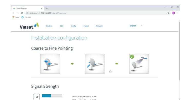
During the Point and Peak process, the Modem Browser Interface records the current and the peak RX SNR levels in the Signal Strength section. These two levels will match when an antenna is aligned correctly.
