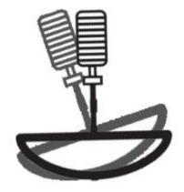
Sweep the antenna toward the left, listening for the TRIA to emit the low/slow tone, which means that the antenna has found the far edge of its frequency set.
