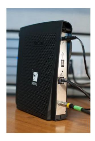
Connect the COAX cable between the Transmit (TX) port on the TRIA, and the TX port on the SB2 modem.
