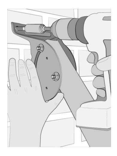
Hold the level along the side flange or the top of the footplate, and slide the footplate side to side until the horizontal bubble is centered. When the footplate is level, mark the wall in the remaining three outside holes of the footplate. The center holes are not used because they will likely align over the mortar. Pre-drill the outside holes of the footplate as before.
