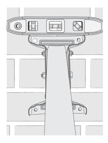
Use a hammer to insert one expansion anchor into each hole. To secure the other three corners, use  $5/16 \times 2$  inch flanged lag screws
