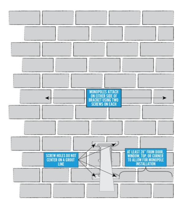
Hold the footplate in the center of the brick and mark the top-left outside corner hole. Remove the footplate and use a concrete drill bit to drill a  $\frac{1}{2}$  inch hole on the mark.
