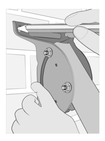
After pre-drilling, hammer the double expansion anchor into the hole, ribbed end in first, until it is flush with the surface of the base material.
