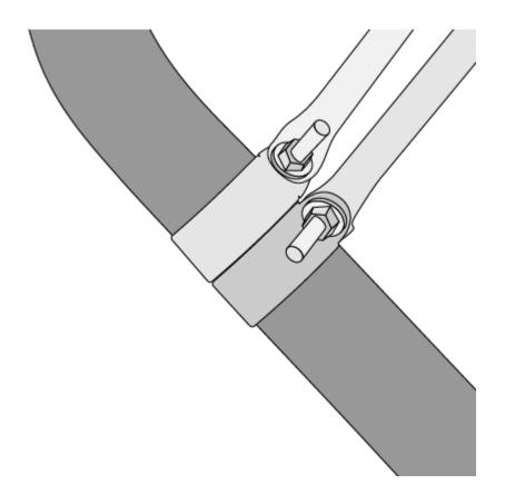
Position the monopoles 9 to 13 inches from the top edge of the footplate, which should put the monopoles at an angle of  $60^{\circ}$  to  $65^{\circ}$  from the tube as shown.
