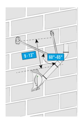
Using the same technique and process as the footplate, attach the foot of each adjustable monopole to the wall using 2, 5/16 X 3 inch lag screws per foot.
