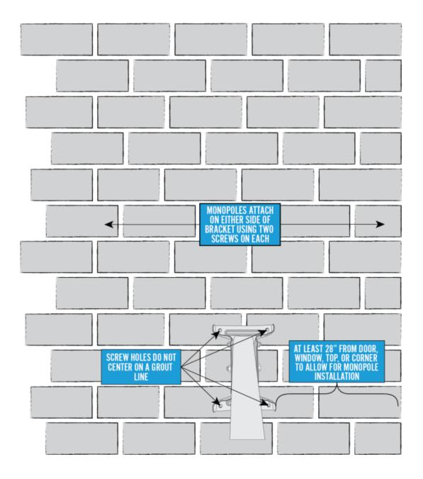
Hold the footplate in the center of the brick and mark the top-left outside corner hole. Remove the footplate and use a concrete drill bit to drill a  $\frac{1}{2}$  inch hole on the mark.
