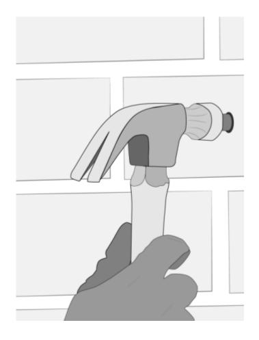
Place the footplate on the wall, aligning the top-left outside hole with the hole in the wall. Add a silicone-based sealant, and then secure with a  $5/16 \times 2$  inch flanged lag screw
