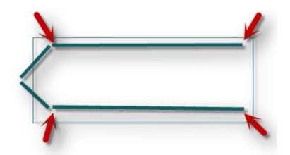
An I-beam Clamp on a structure's main metal frame can provide ground on **mobile homes only**. When grounding to a mobile home, install the clamp **at the end of the I-beam**. Never install the clamp in the middle or the front angled part of the frame, or on the straps that surround the beams.
