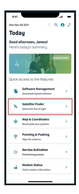
Press the correct satellite and use the mobile camera to locate the satellite. Before entering an area with no service, Satellite Finder will easily let you find the satellite in space. From your position on site, simply follow the prompts.
