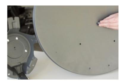
After mount installation is complete, place the antenna on the mast.
