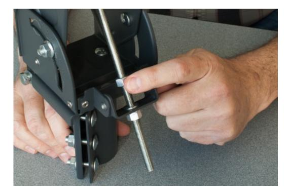
Manually adjust the elevation setting to the relevant position by turning the Elevation Adjustment Nut.
