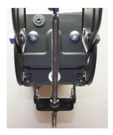
Once the azimuth is centered, retighten the bolts on the bottom of the AZ/EL assembly to secure the setting while the antenna is being built.
