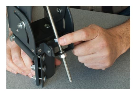
Manually adjust the elevation setting to the relevant position by turning the Elevation Adjustment Nut.
