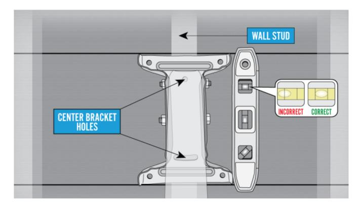
After removing the footplate, use these marks to drill the remaining five 1/8 inch holes; one in the center bottom and one in each outside corner.
