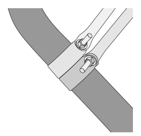
Position the monopoles 9 to 13 inches from the top edge of the footplate to the 2 adjacent wall studs, which should put the monopoles at an angle of  $60^{\circ}$  to  $65^{\circ}$  from the tube as shown.
