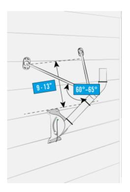
Using the same technique and process as the footplate, attach the foot of each adjustable monopole to the structural element (stud) using 2,  $5/16 \times 3$  inch lag screws per foot.
