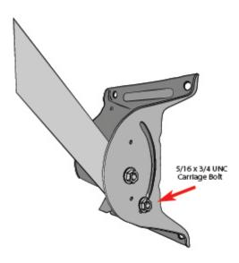
Swing the mast tube up and use a level to level the mast tube. Tighten the footplate carriage bolts to ensure the mount is plumb. Complete final mast tube leveling after installing the monopoles.
