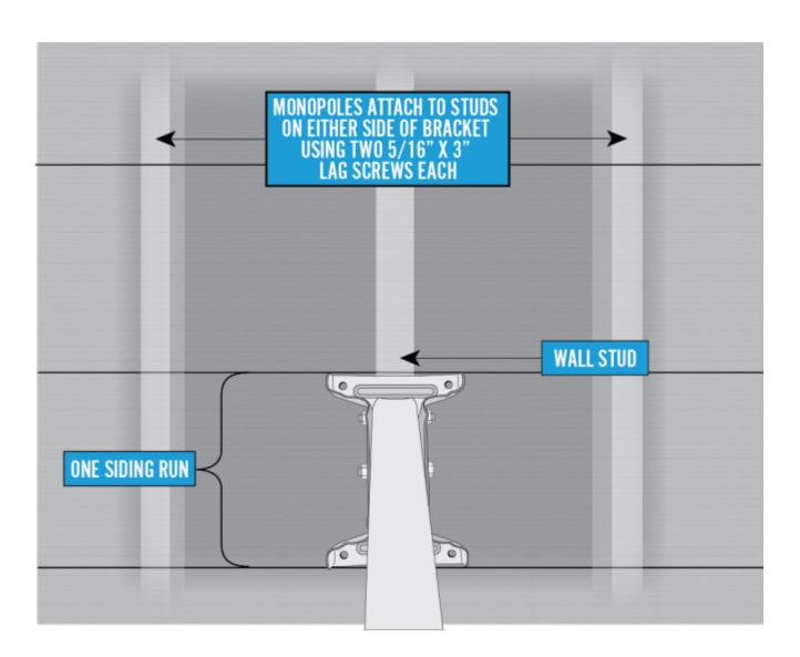
Hold the footplate in the center of the stud and mark the topcenter hole. Remove the footplate and drill a 1/8 inch hole on the mark.
