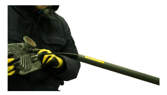
Attach the replacement TRIA to the boom arm
