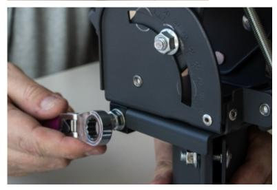
Turn the Fine Azimuth adjustment nut until the indicators on the base of the AZ/EL are at Zero (0).
