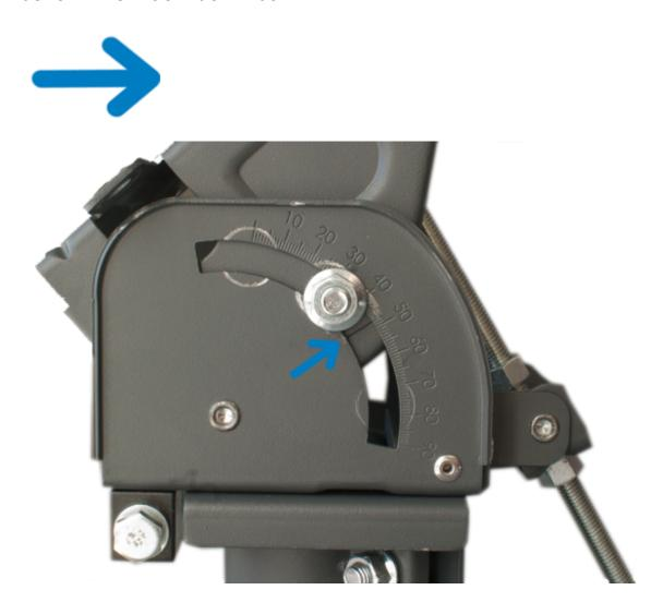
When the coarse elevation adjustment is complete, wind the top nut down the elevation rod until it bottoms out on the cast pivot bracket. Tighten the elevation lock down bolts on the AZ/EL assembly. This will secure the setting while the antenna is being built.
