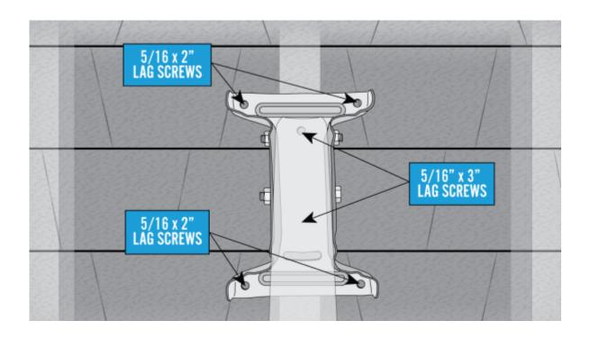
Correctly align the footplate over the 1/8 inch holes. This will allow correct placement directly over rafters or trusses.
