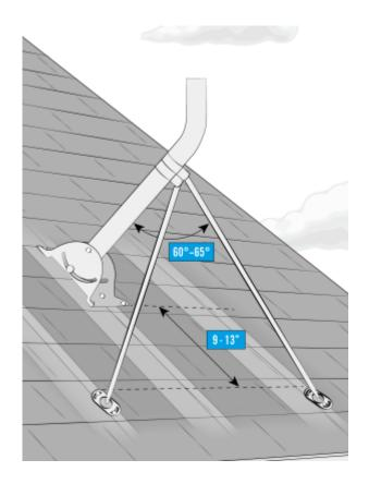
Using the same technique and process as the footplate, attach the foot of each adjustable monopole to the structural element (rafter) using 2, 5/16 X 3 inch lag screws per foot.
