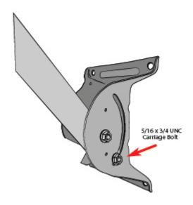
Swing the mast tube up and use a level to level the mast tube. Tighten the footplate carriage bolts to ensure the mast is plumb. Complete final mast tube leveling after installing the monopoles.
