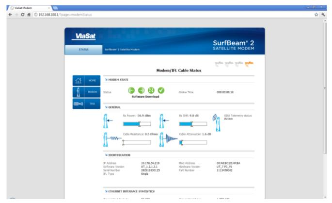
After the modem obtains modem lock, the status indicator reads 'Online.' If a software download is available, the indicator's label changes to read 'Software Download.'
