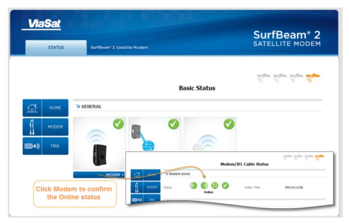
At the end of the Point and Peak process, the right arrow was clicked to have the modem attempt Modem Lock. When the modem has locked, the Modem Browser Interface will show 3 green checkmarks.
