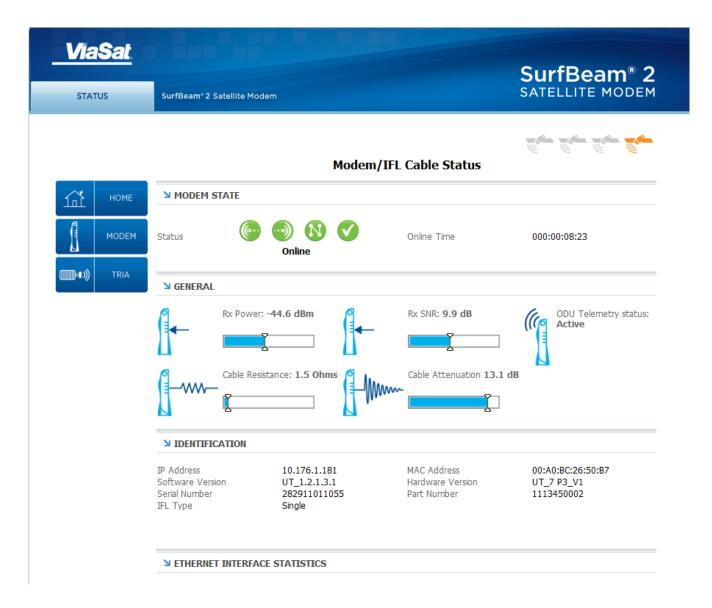
If the modem fails to lock (online status indicator), then put the modem into Install Mode using this URL: 192.168.100.1/install. Return to the antenna and complete a Push/Pull Test, and attempt Modem Lock again. Continue to follow the TIC until the modem locks, if necessary.
