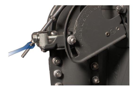
Sweep the nut on the Elevation rod such that the TRIA drops, and listen for the TRIA to emit the low/slow tone, which means that the antenna has found the far edge of its frequency set. Stop, as this is the end of the first fine-tune learning pass.
