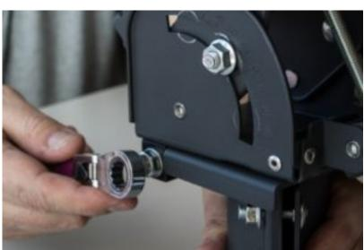
Rotating the hex head beyond the low/slow tone during the peaking procedure can compress the bolt's attachments, causing them to fail.
