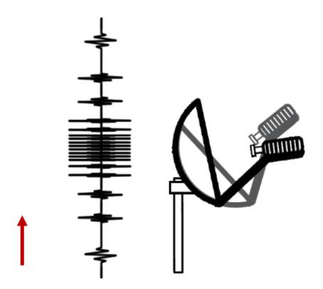
Reverse the direction of the sweep again, now sweeping to the center, and listen for the TRIA to emit the high/steady tone. The antenna is now in the center of the beam.
