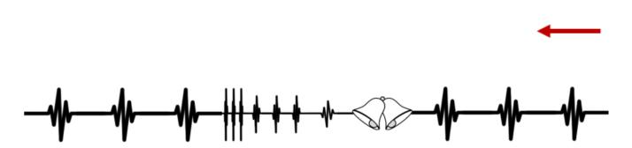
Reverse the direction of the sweep, and listen for the TRIA to progress through the tone sequence. Stop the sweep when the TRIA emits the heartbeat tone. This is the end of the second learning pass.
