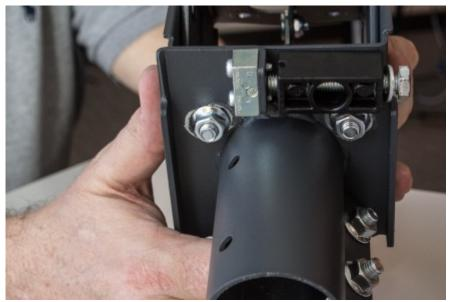
Using an open wrench, rotate the hex head of the Azimuth fine-adjust bolt.
