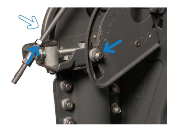
Use the open wrench on the lower Elevation rod nut.
