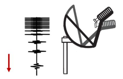
Reverse the direction of the sweep, now sweeping to raise the TRIA, and listen for the TRIA to progress through the tone sequence. Stop the sweep when the TRIA emits the low/slow tone. This is the end of the second fine-tune learning pass.
