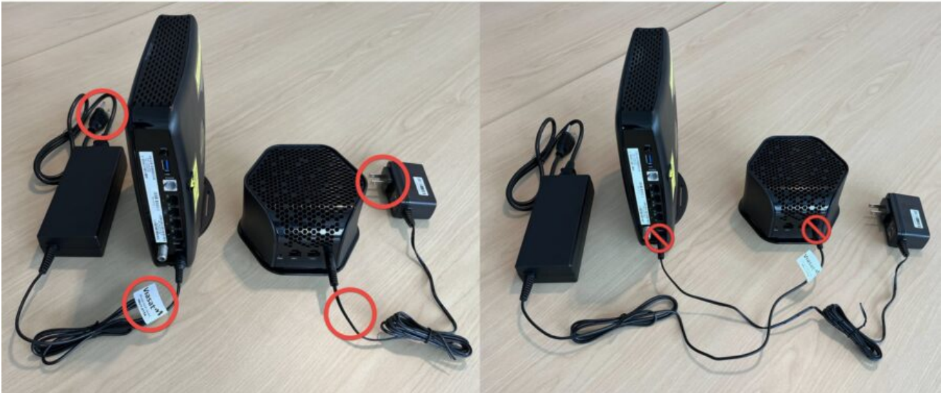
Correct / Incorrect power cord installation
