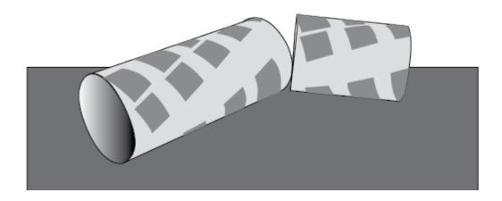
3. Place the 3 foot concrete form tube in the hole with 1 inch hole toward bottom. Tube will extend 12 inches above ground level
