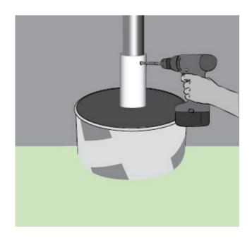
14.Place  $\frac{1}{4}$  inch x 6 inch bolts, washers, and nuts through holes Tighten  $\frac{1}{4}$  inch nuts until telescoping pole is secure
