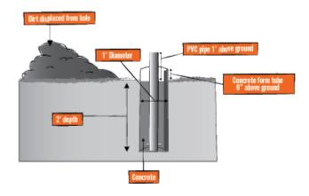
2. Concrete form tubes with a 8 inch inside diameter come in standard 4 foot sections
