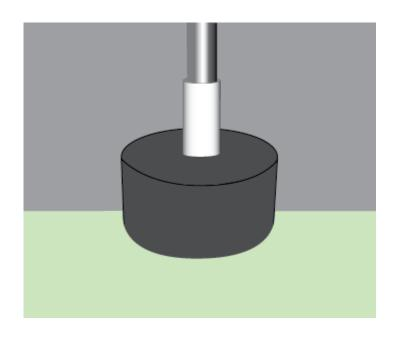
12. Ensure that the SXT faces the direction of the Base Station, for point-to-point signal
