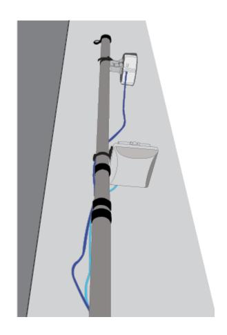
10. Mount the weatherproof (NEMA rated) enclosure a minimum of 7 feet above ground level, with 2 self-tapping screws
