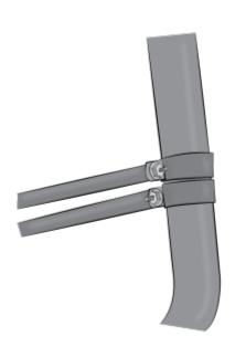
Using the same technique and process as the footplate, attach the foot of each adjustable monopole to the structural element (fascia) using 2,  $5/16 \times 3$  inch lag screws per foot.
