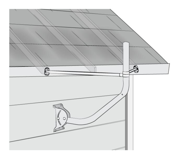
Hold the footplate in the center of the structural element (stud) and mark the top and bottom center holes. Remove the footplate and predrill 1/8 inch holes on the two marks.
