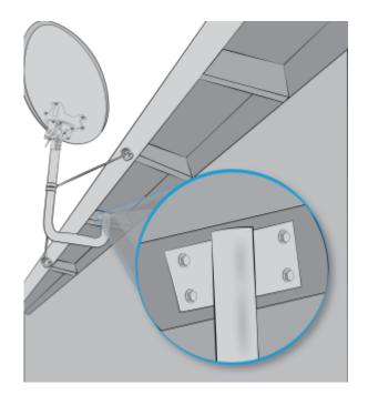
Locate the structural elements (rafters) that will place the footplate in position to meet all of the appropriate considerations listed above. Do not forget to allow room for the adjustable monopoles.
