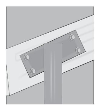
Correctly align the footplate over the 1/8 inch holes in the rafter. Fill the holes with silicone-based sealant.
