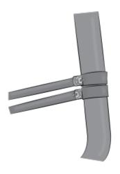
Using the same technique and process as the footplate, attach the foot of each adjustable monopole to the structural element (rafter) using two  $5/16 \times 2$ -inch lag screws per foot.
