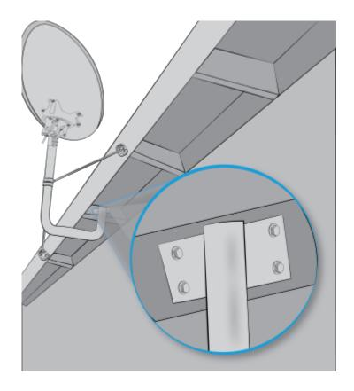
Tighten all the 5/16 inch hardware joints.
