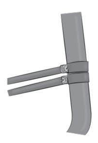
Using the same technique and process as the footplate, attach the foot of each adjustable monopole to the structural element (rafter) using two  $5/16 \times 2$ -inch lag screws per foot.
