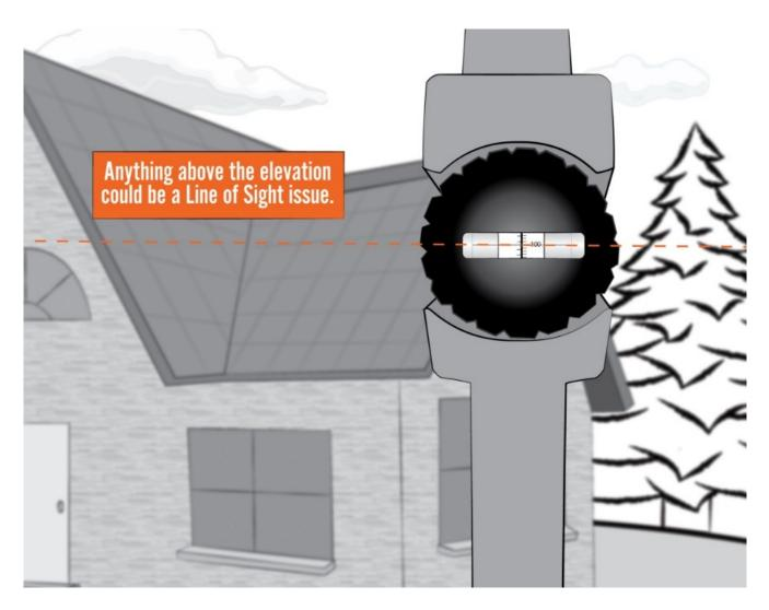
Once you have determined that the LOS is clear, begin installing the antenna
