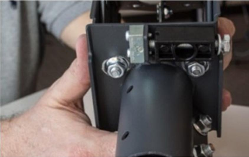
Using an open wrench, slowly turn the Azimuth fine-adjust bolt, listening for the pTRIA to emit the '**low/slow**' tone. This means that the antenna has found the far edge of its frequency set.
