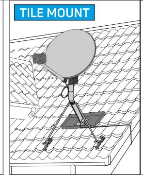
Attach to an approved, structurally sound surface on a sloped tile roof (clay or concrete tiles only)
